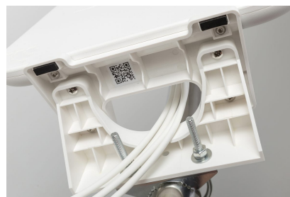
Frame to antenna. Four M4 × 8 screws; cables exit the centre.
