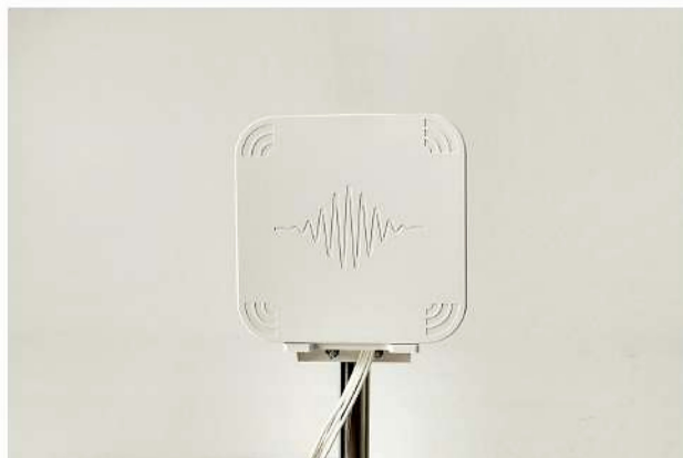
Pole mount. The support frame holds the antenna clear of the mast on poles up to 50 mm in diameter — the usual choice for outdoor and roof installations.
