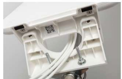
Frame to antenna. Four M4 × 8 screws; cables exit the centre.
